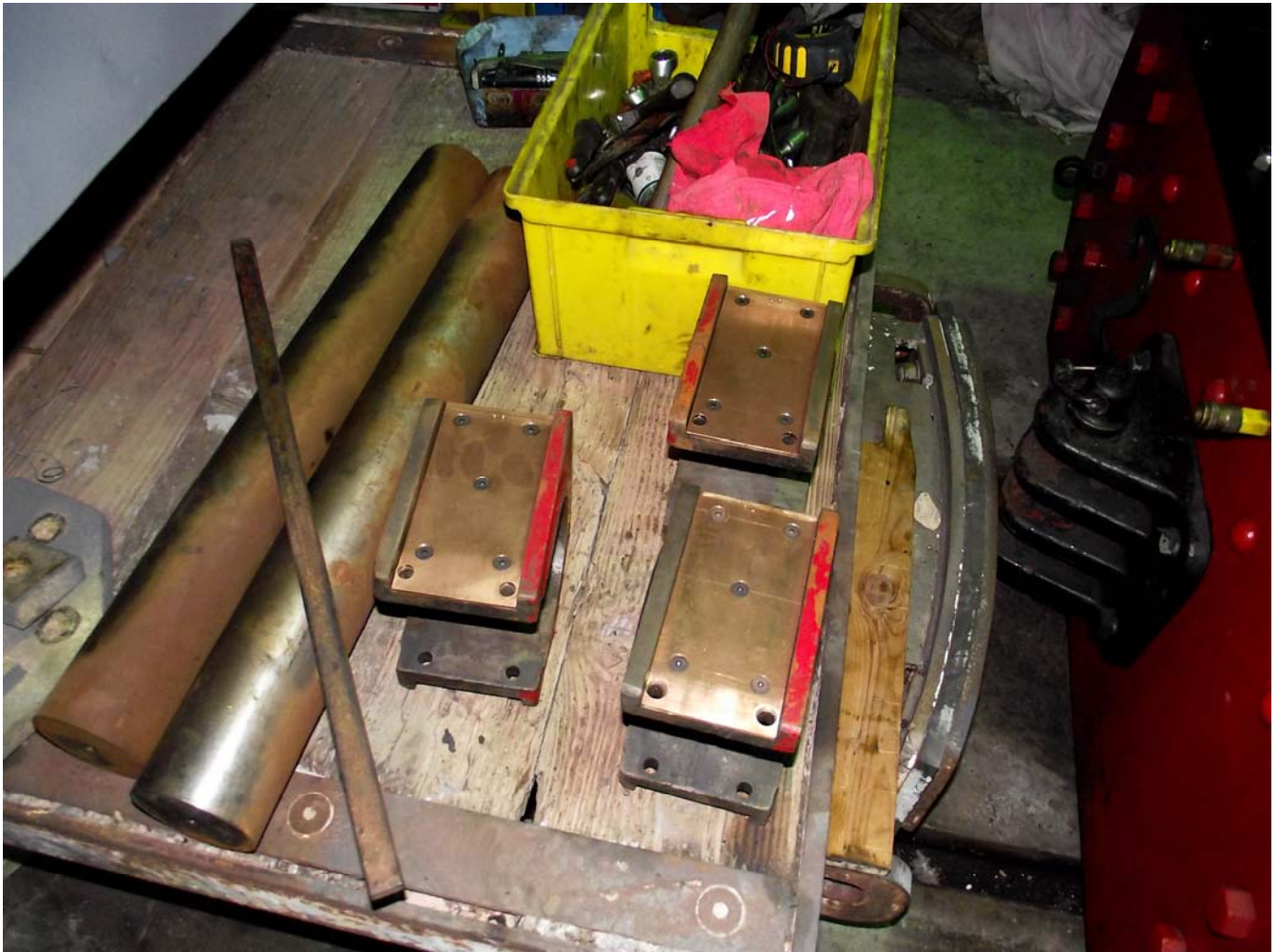
The new bronze shims to three of Lorna Doone's axleboxes, awaiting final machining
