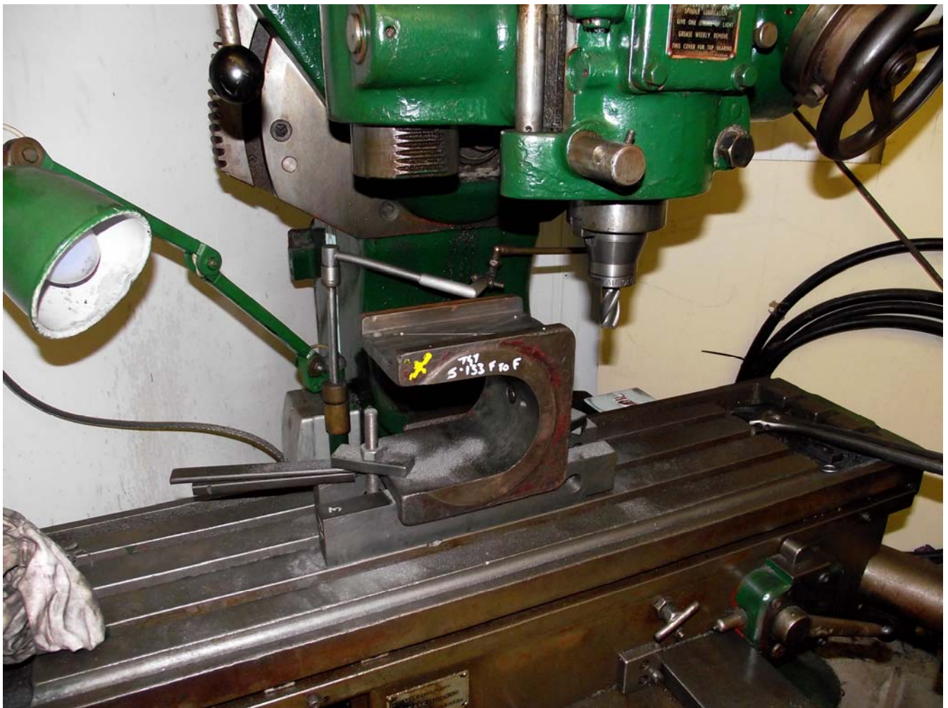
One of Lorna Doone's axleboxes set up on the Archdale mill
