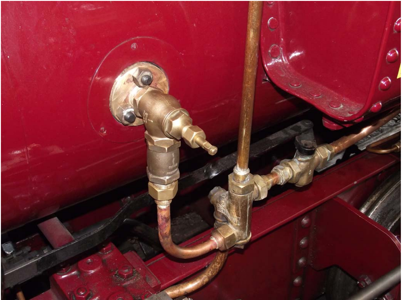
Jennie's new driver's side clack, note the screw down valve
