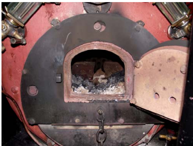
Isabel's firebox with the collapsed brick arch, since replaced
