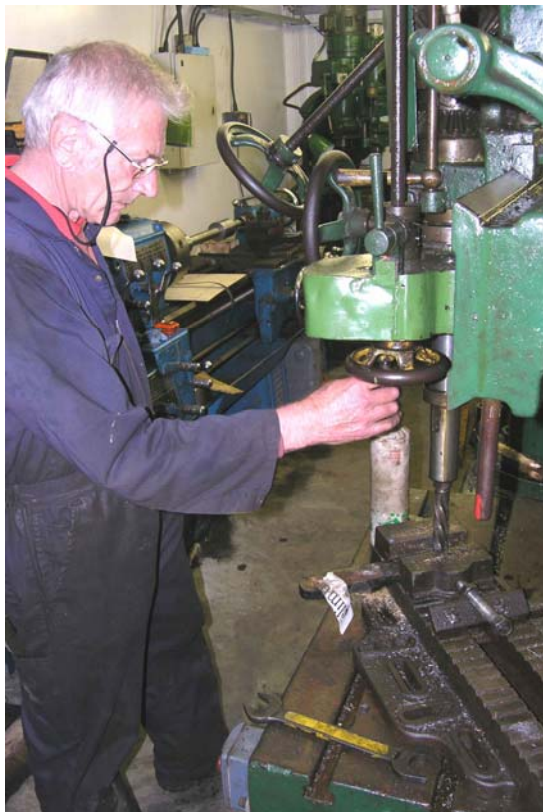
Work continues on Lorna Doone by machining brake parts on our radial arm drill
