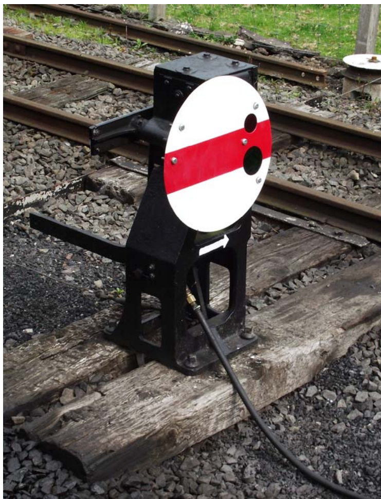
Refurbished dolly signal in the loop at Amerton
