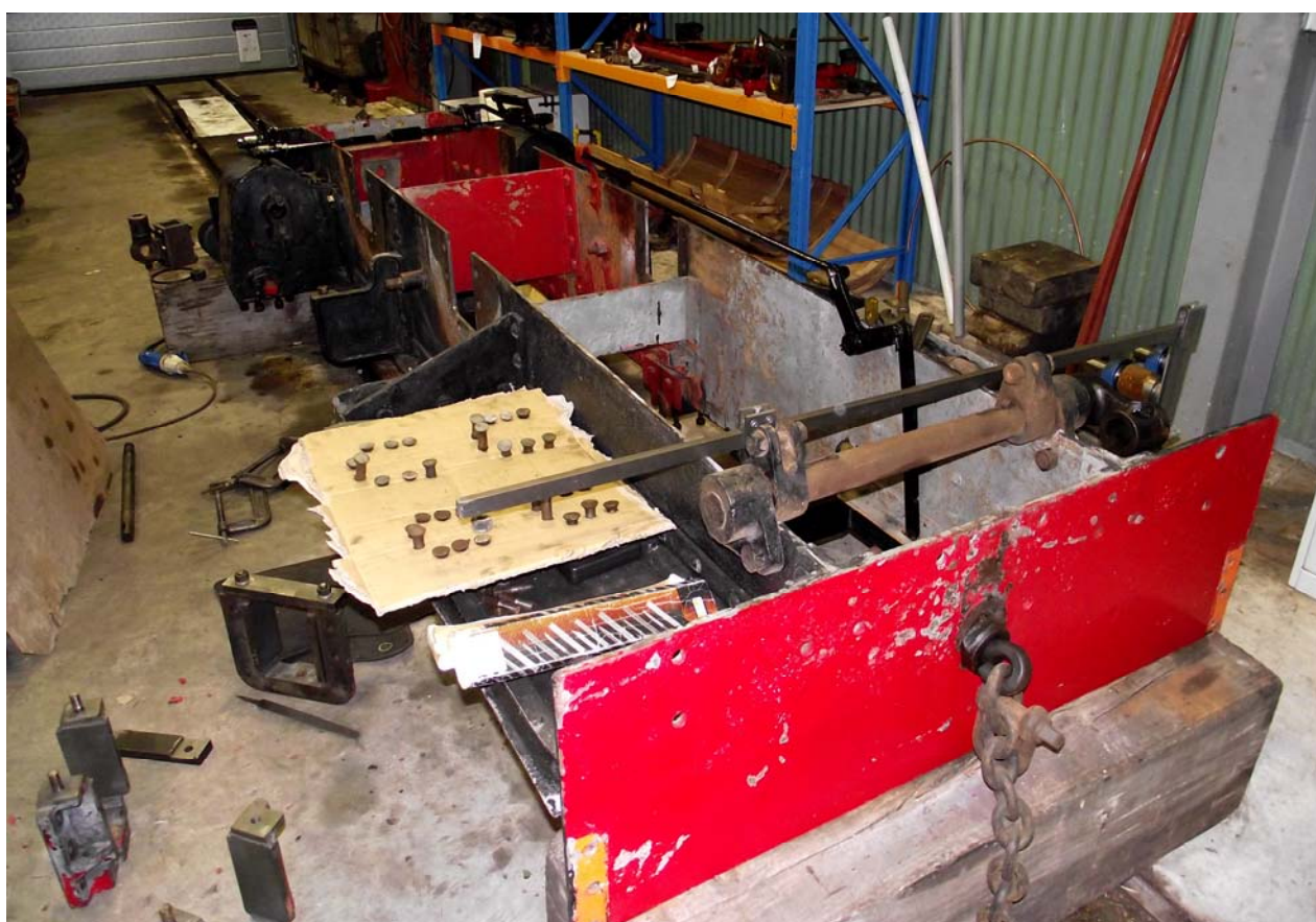
Lorna Doone's frames upside down and prior to shotblasting
