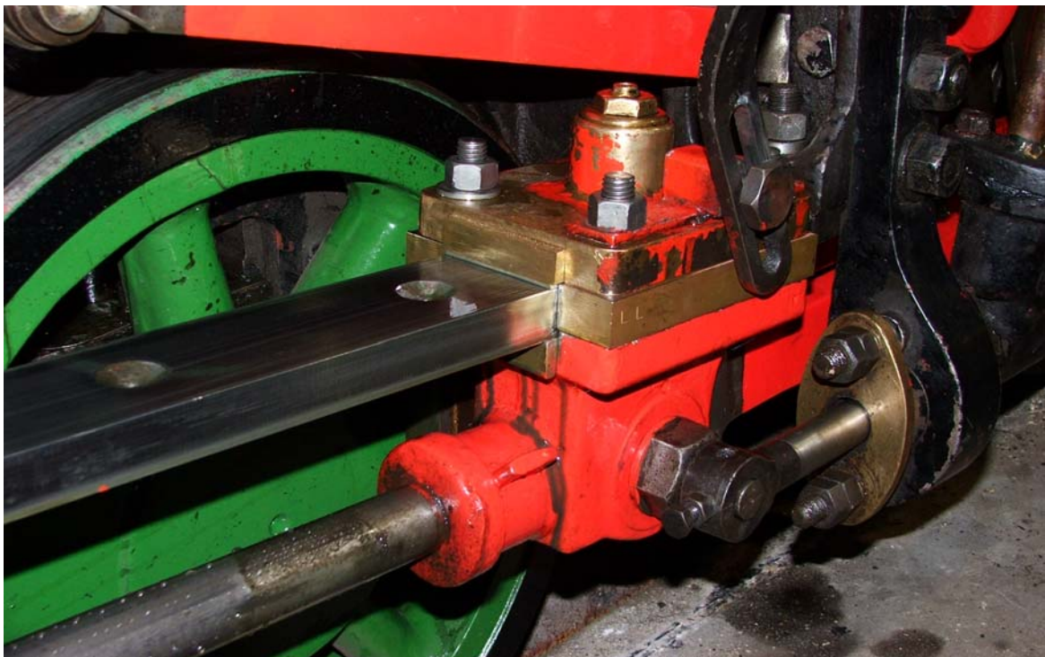
Isabel's completed crosshead showing the new top and bottom white metal lined slippers
