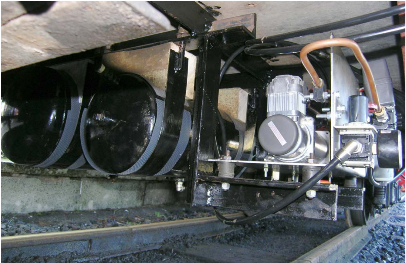
Air tanks, regulator and compressor (on right) mounted underneath No 1 coach
