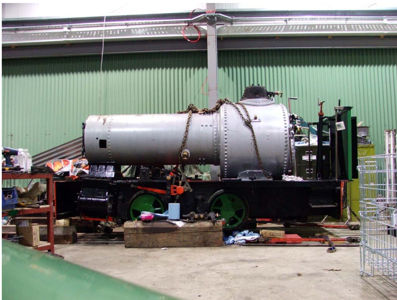
Isabel's new boiler is tried in the frame for the first time! It kind of fits!
