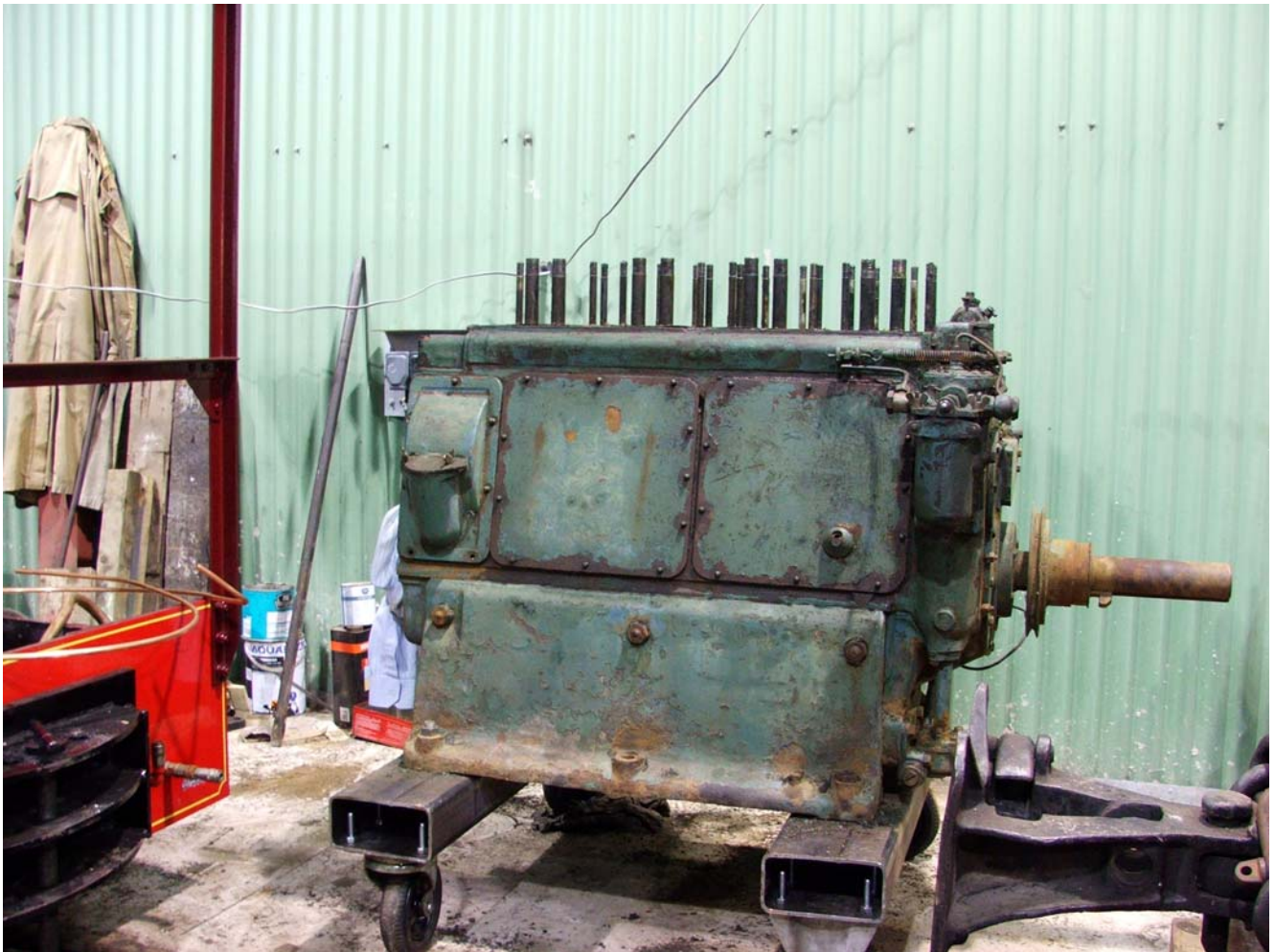
The ex Gen Set Ruston 4VRO set up on the new trolley, with heads removed just prior to full dismantling John Strike
