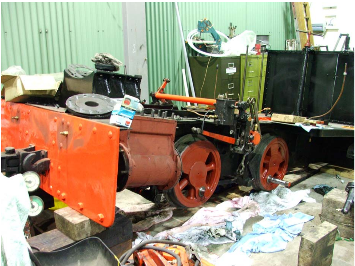
Isabel's frames jacked up and having the drain cocks refitted and primer applied to the wheels
