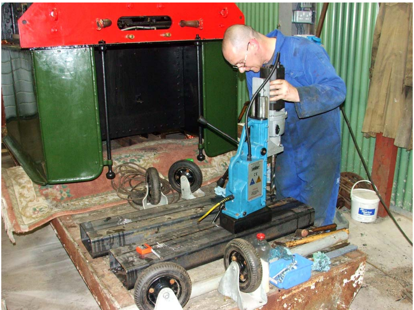
Nick drills the fixing holes for the heavy duty castors for the Ruston 4VRO trolley
