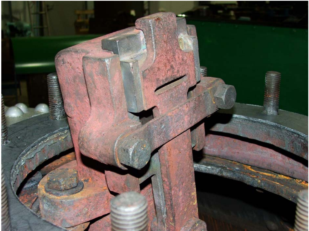
Close up of Isabel's regulator valve; note that the pilot valve drags the main valve open
