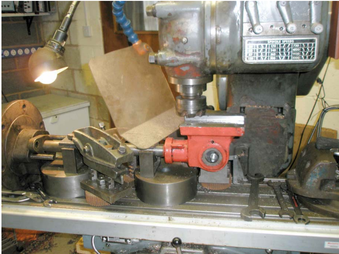
Machining Isabel's crosshead ready to receive a new slipper
