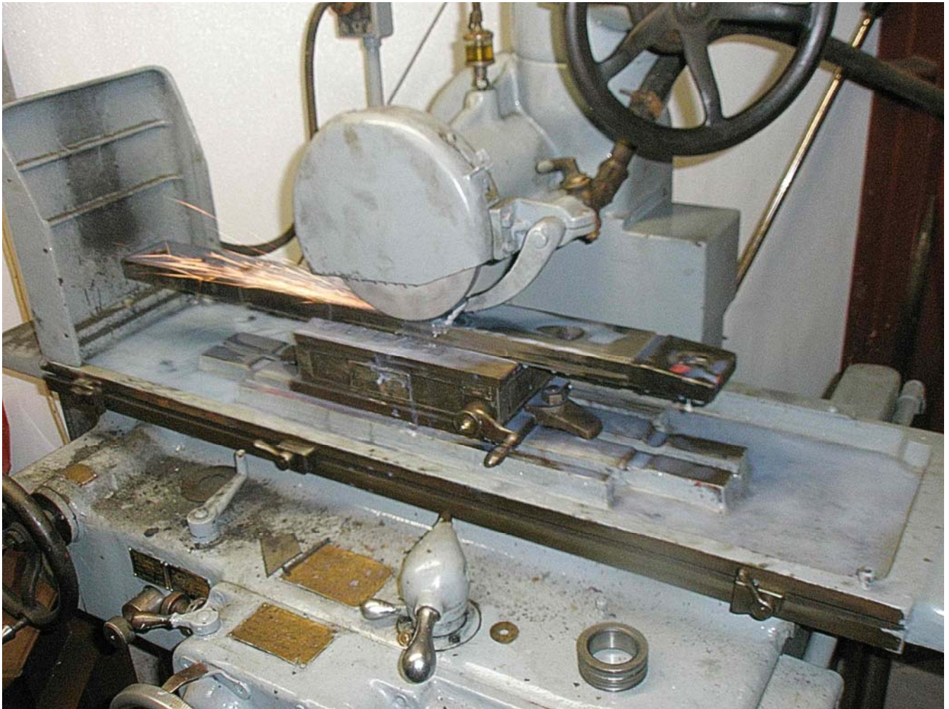
Surface grinding Isabel's slidebars
