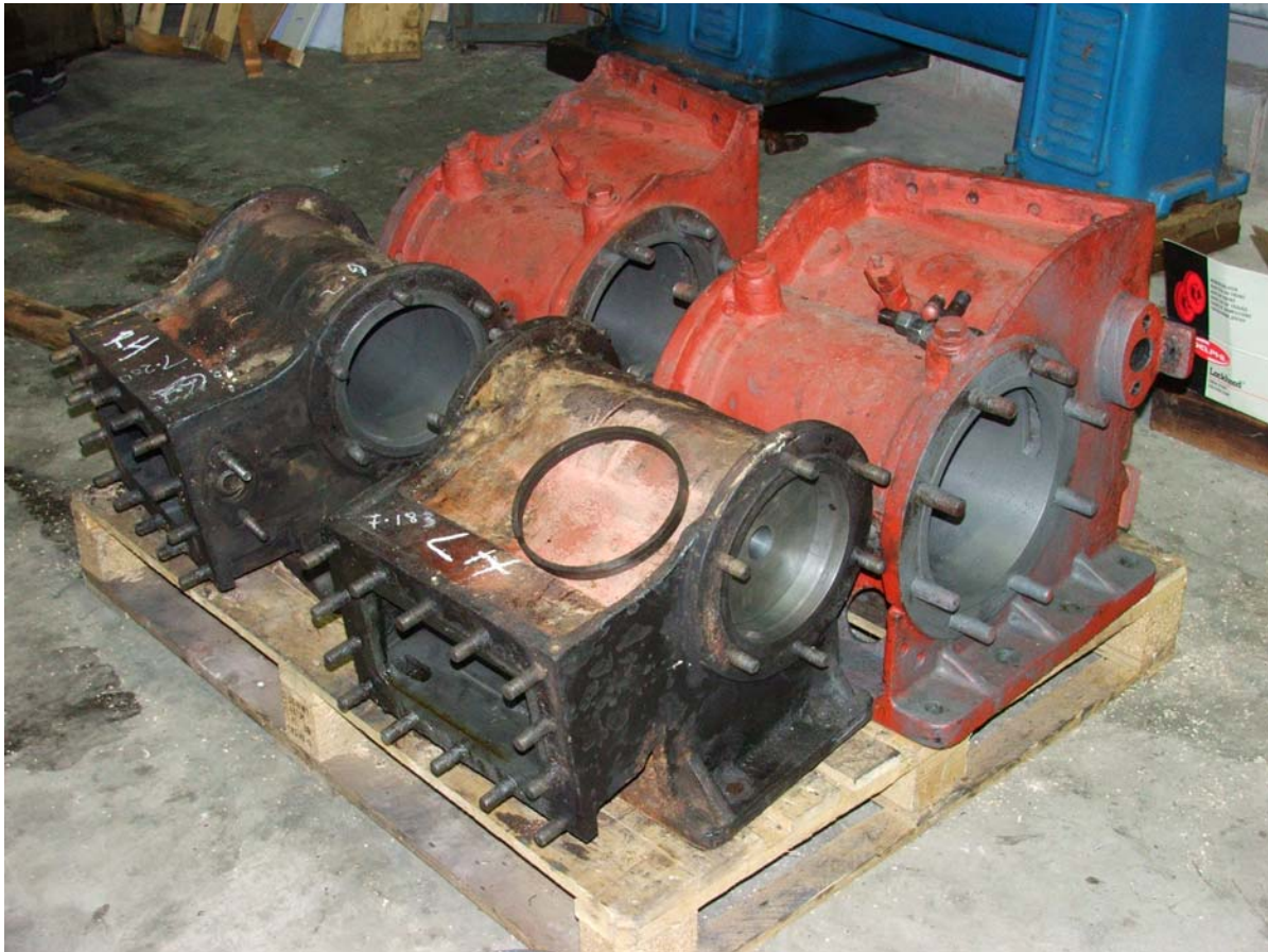
Machined cylinders, Isabel's on the LHS, Henschels on the RHS, note the difference in size! John Strike
