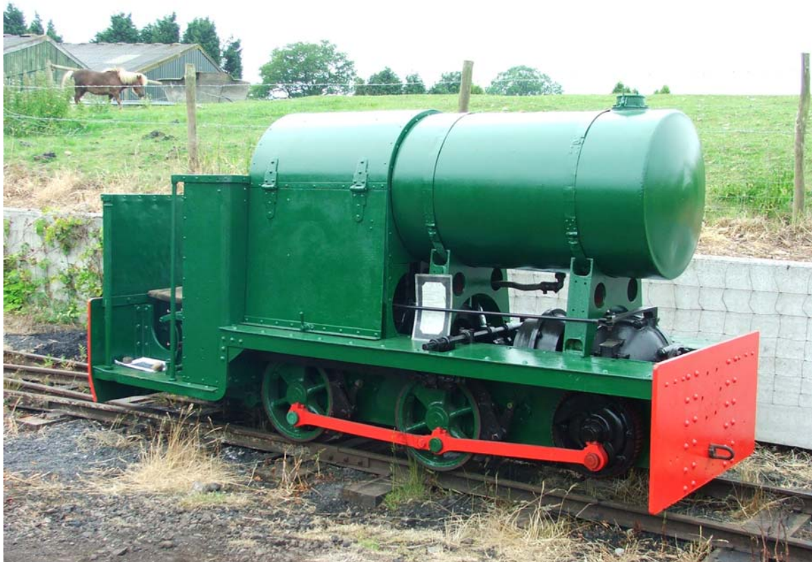
20hp Baguley 0-4-OPM number 774 on display for the first time
