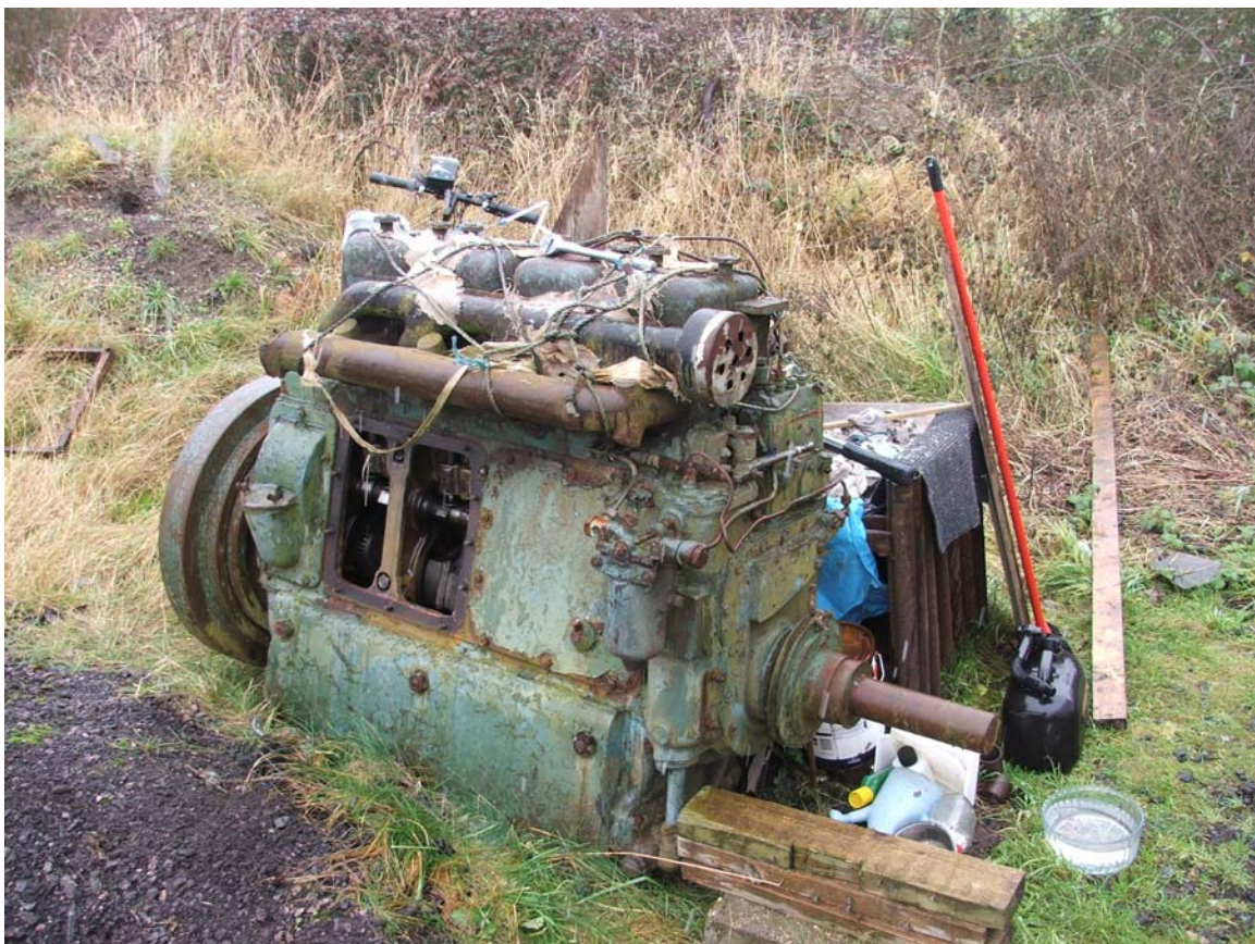
The ex Second World War gen-set 4VRO with inspection cover removed
