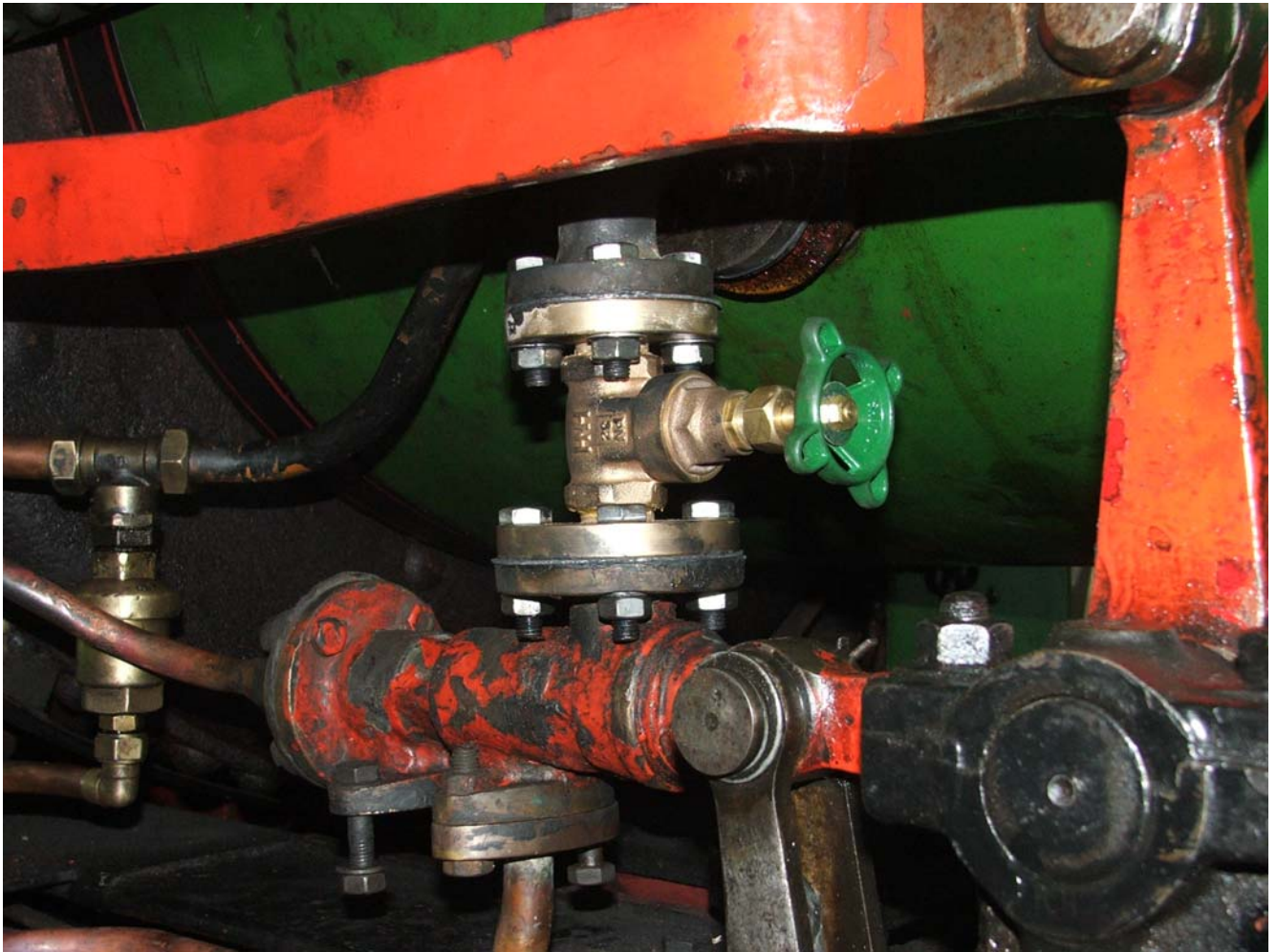
The new isolating valve between the injector and the clack on Isabel
