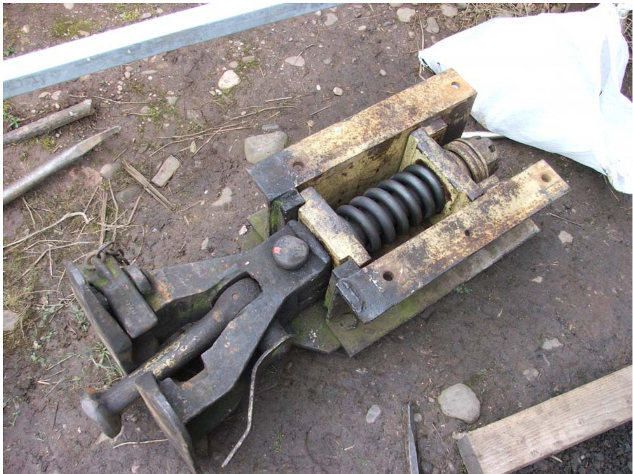
The new spring as fitted to the Allens coupling housing
